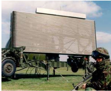
Figure 23. Commander AR327 - Type 101 air defense radar
