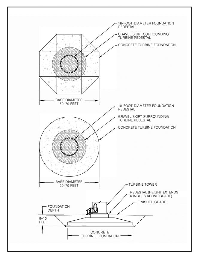
Figure 2.3-5. Typical Wind Turbine Generator Footing Foundation
