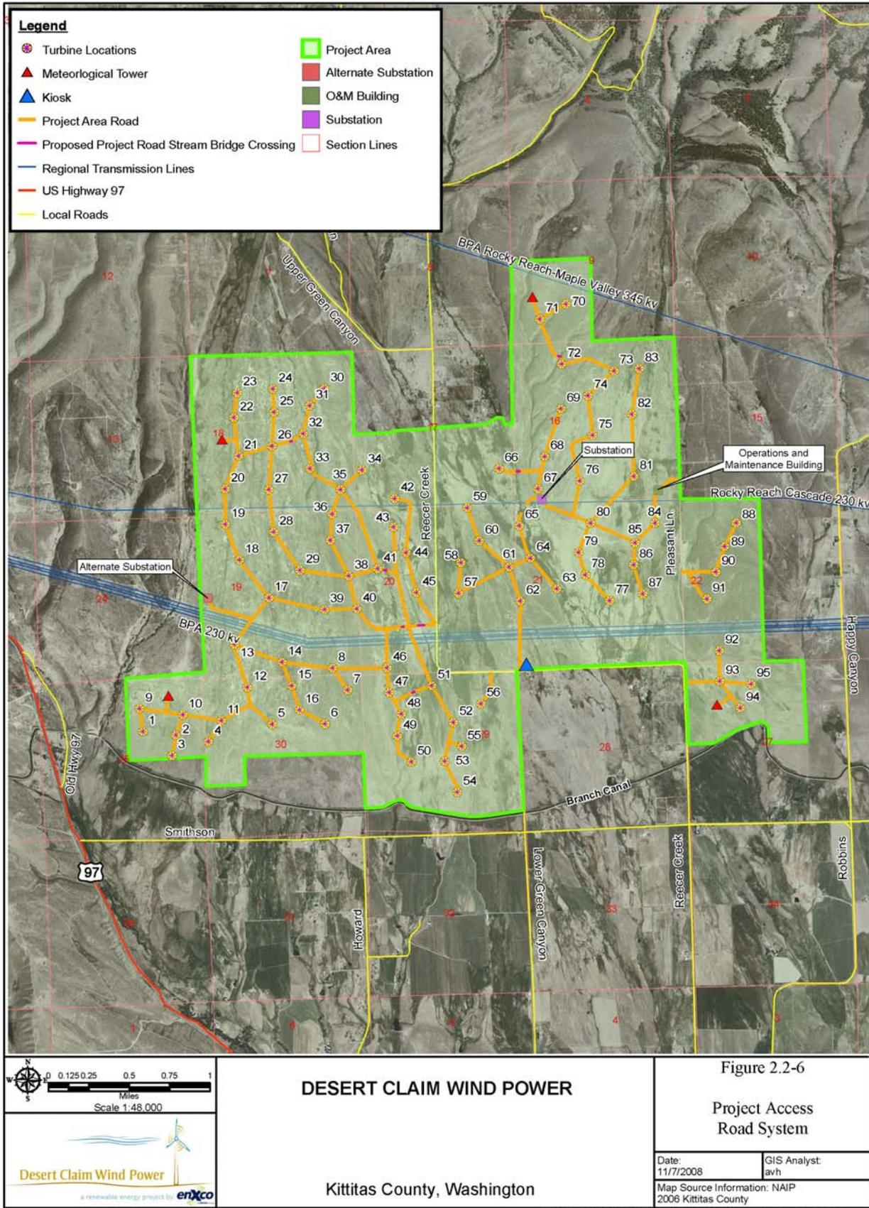
Detailed plans for the Project road system and the connections to county roads would be prepared following micro-siting of the turbines. Project access road connections to county roads would be designed pursuant to County road ingress and egress standards.
