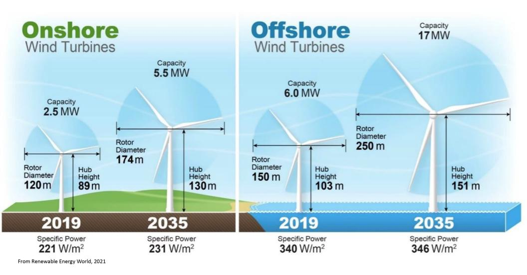
Taller turbines reach further into the atmosphere where it is more stable and wakes recover more slowly. Neutral and unstable atmospheres are more common near the surface, but overall are more rare than stable. Stability varies continuously.
