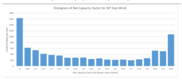
Referring to the chart - if you sum up the number of MWhs produced by multiplying the hours times the capacity factors times the nameplate rating (assume 1 MW for simplicity) and divide that by the total yearly hours (8760) you see that only 42% of MWh capacity was produced. Firm Transmission requires 100% of nameplate MW, but only 42% of MWhs would be loaded, meaning the transmission line was 58% inefficient with respect to its MWh capacity. How can this be addressed?
