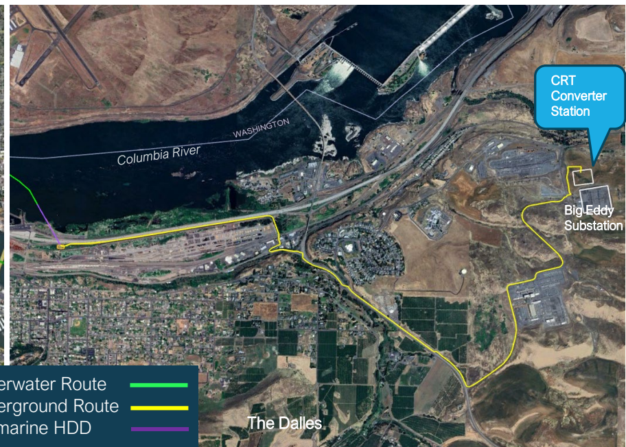
The Dalles 5-mile Underground Line
